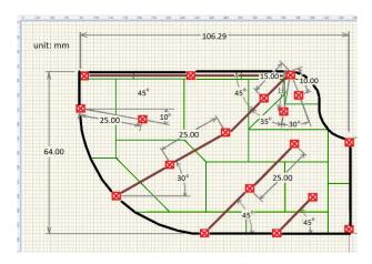
Fig. 2. Flapping wing partition of "Golden-Snitch".
