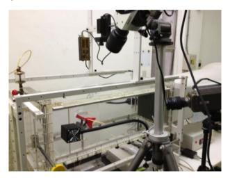
**Fig. 3.** The 3D trajectory experiment set up with 2 high-speed cameras.
